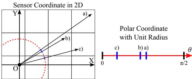
Fig. 1. This figure shows an observation that rays, associated with adjacent points in the polar coordinates, traverse a similar set of cells. The three rays –  $a)$ ,  $b)$ , and  $c)$  – starting from the sensor origin  $O$  are mapped onto a unit circle represented by red dotted circle. In the polar coordinate, the mapped points associated with the three rays are shown as the blue lines.
