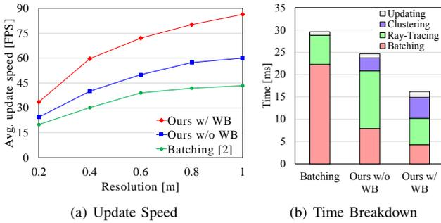
Fig. 3. These figures show performance of updating an octree-based occupancy maps in the dataset using 8-threads. We measure the average performance according to various resolutions for different methods in figure a). Also, we report the average breakdown of the total time taken for updating the map with 0.6m resolution in figure b). WB indicates our workload balancing method.
