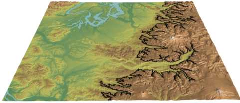
Fig. 5. Puget Sound Iso-contour: The contour line (in black) at 720 m elevation was extracted from an unstructured terrain model consisting of 134M triangles. The contour passes through 286K triangles.
