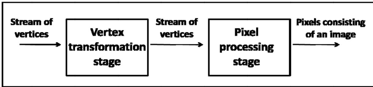
Since these two stages can be performed independently, we can perform these two stages in a parallel manner in graphics hardware. For example, after performing vertex transformation to  $v_1, v_2, v_3$ , we perform rasterization step for a triangle consisting of those three vertices. During rasterizing the triangle, we can perform vertex transformation to other vertices, say,  $v_4$ .
