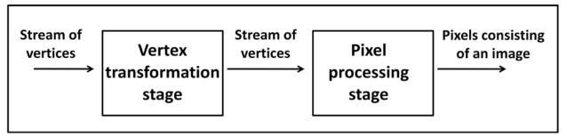
Since these two stages can be performed independently, we can perform these two stages in a parallel manner in graphics hardware. For example, after performing vertex transformation to v1, v2, v3, we perform rasterization step for a triangle consisting of those three vertices. During rasterizing the triangle, we can perform vertex transformation to other vertices, say, v4.
