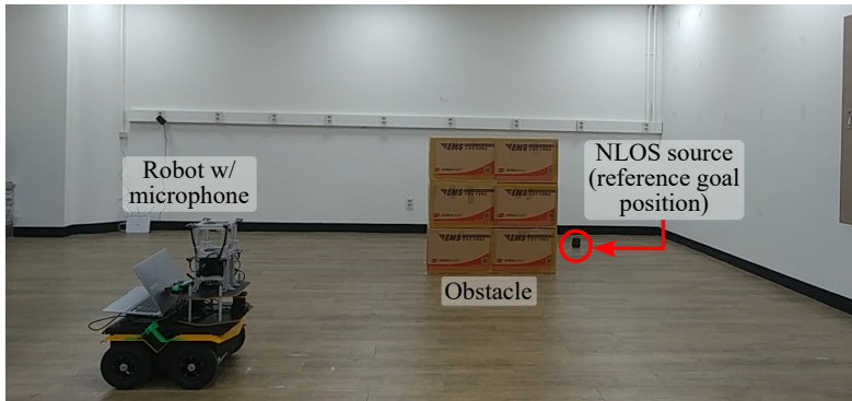
(a) Test environment for navigation to the NLOS case
